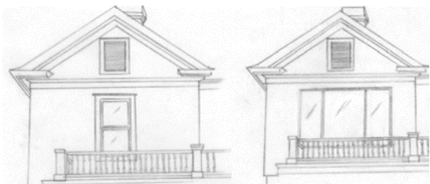
On the left is a good example for replacing a single one-over-one window because the size of the opening and design of the window remains the same. The enlarged opening and fixed windows installed on the right is inappropriate.
